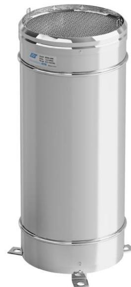
Inside each rain gage is a balanced tipping bucket mechanism with a magnet and switch assembly. Collection of rain is through a 200 mm diameter catchment through a debris filtering screen.
